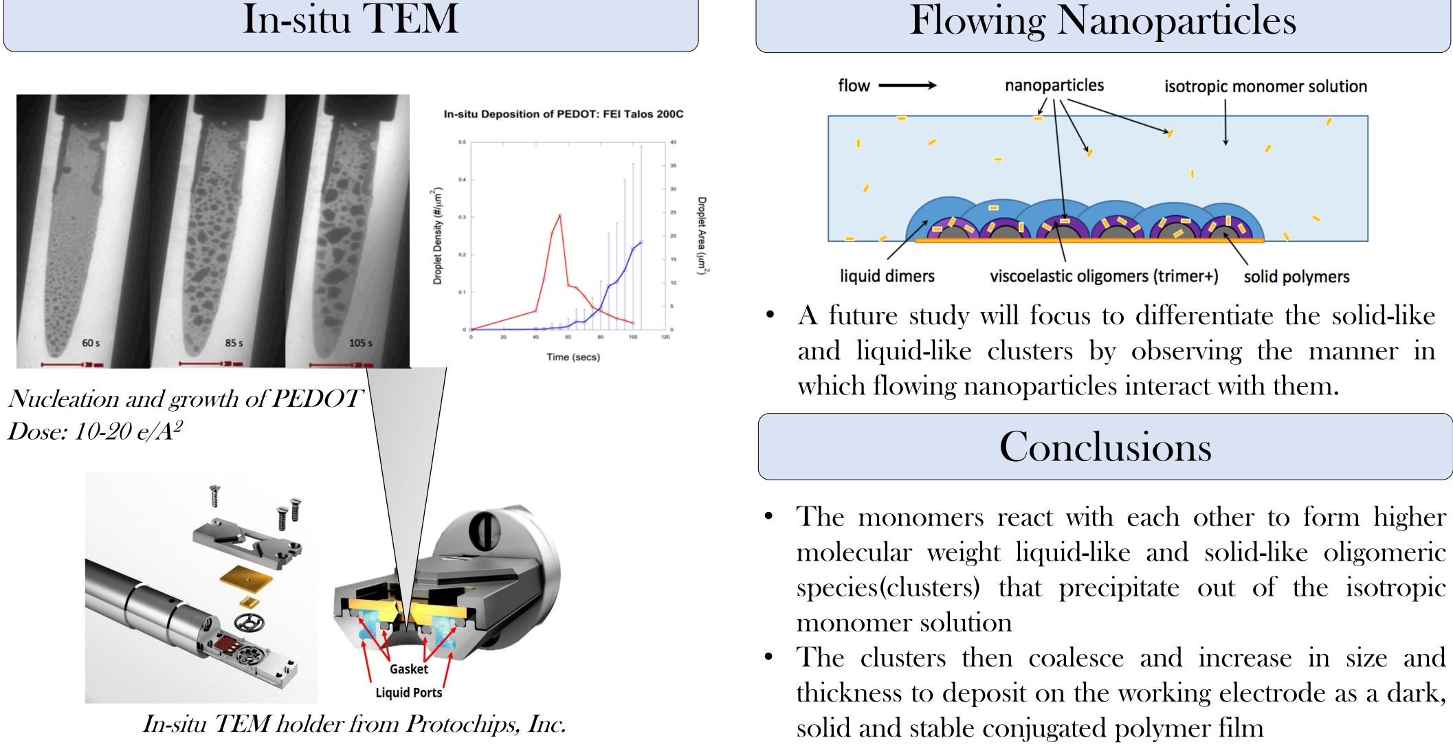
Nucleation and growth of PEDOT with a fibrillar morphology using in-situ TEM (inset: SEM of PEDOT:PAA nanofibrils)
